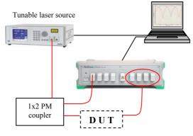
Figure 1: Set up for PM measurement
