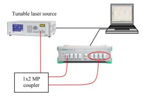
Figure 2: Calibration set up
